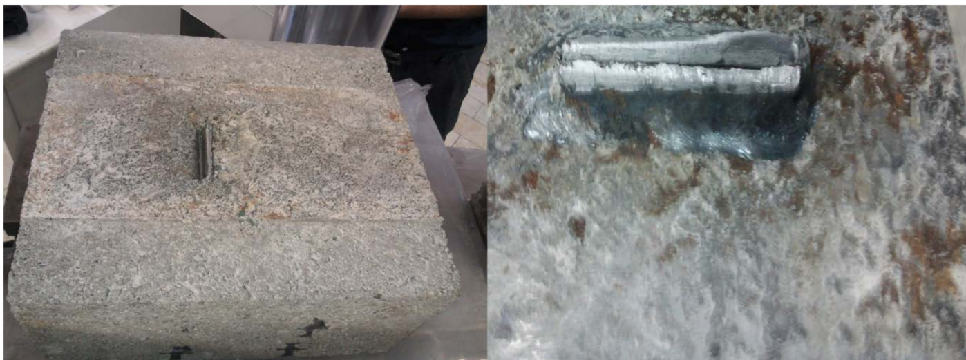
Fig 6. Connector fracture mode (MA112.5L100).
