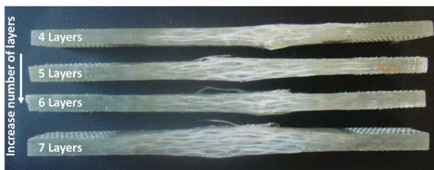
Delamination in failed test samples. Several Vf.
