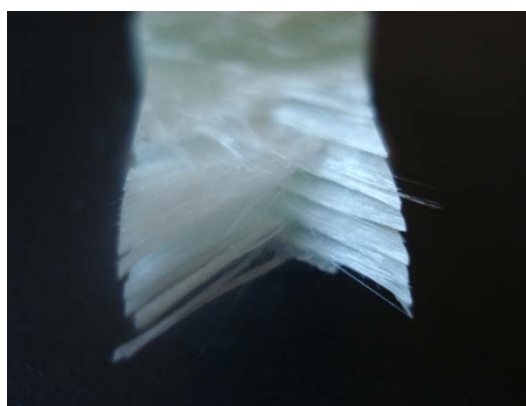
c) Detail of failure of off-axis tests samples , 45^\circ
