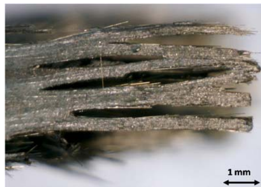
Test sample for 45°, V_f = 36,5, 3,1 \times 10^{-4} \text{ s}^{-1} .
