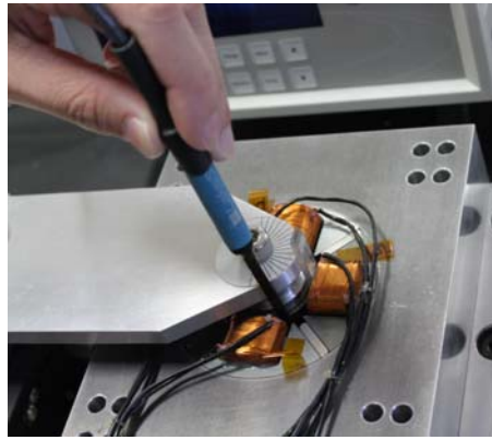
Fig. 12 Fabricated magnetic bearing and flux density measurement
