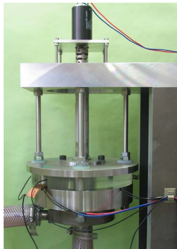
Fig. 18 Photo of magnetically levitated pump
